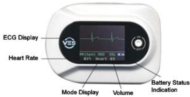
Fig.3-4 ECG monitor interface
